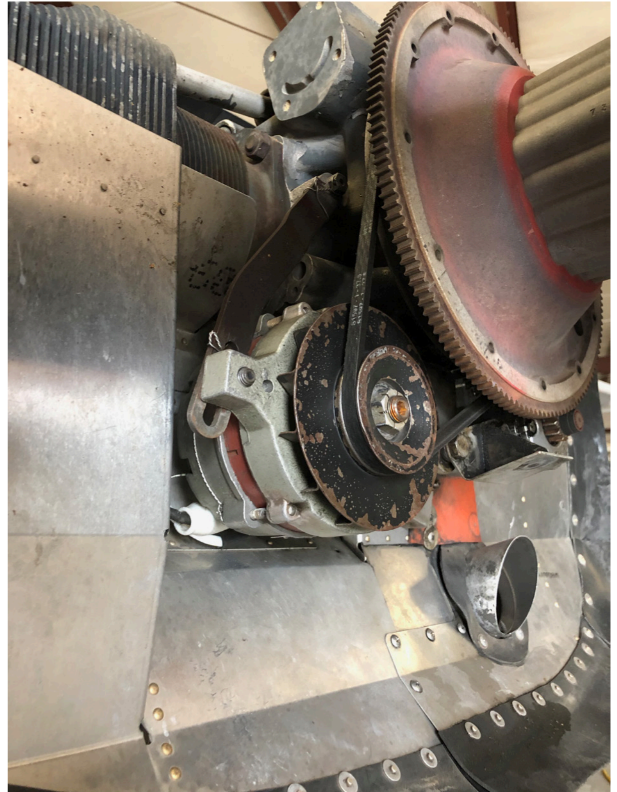
Alternators, such as the one shown here, are most common on modern small airplanes.
