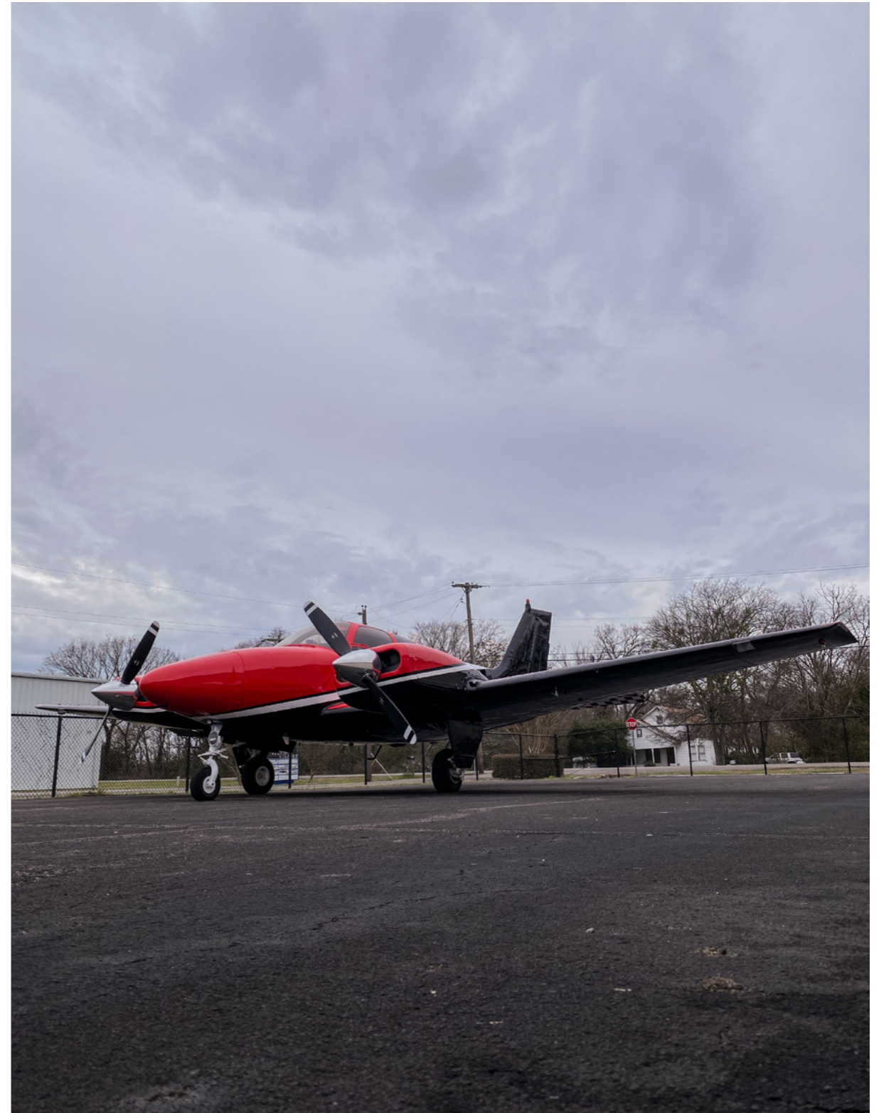
A complex multiengine airplane is required for a commercial pilot AMEL practical test.
